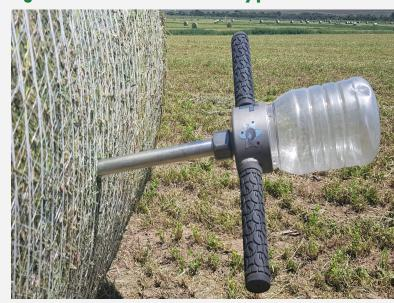
Figure 4.2: Hay probe fitted
